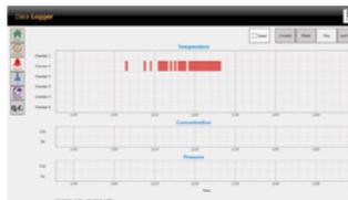
Conditions that put the MIRI® II into alarm state are recorded. It is possible for the software to send email alerts as well.
